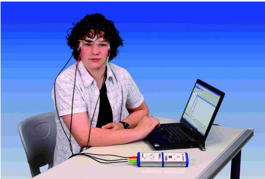
Electrooculogram (alternating eye movements from the left to the right, and vice versa).
