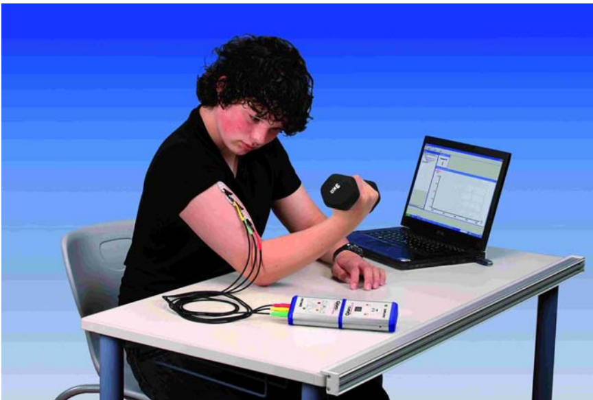
Compound action potentials of the biceps under load by 5-kg dumbbells, as measured on the skin surface. At the end of this measurement, the biceps was not exhausted.
