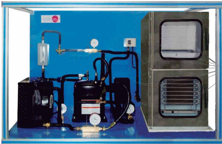
① Unit: TRRC. Refrigeration Unit with Refrigeration and Freezing Chamber
