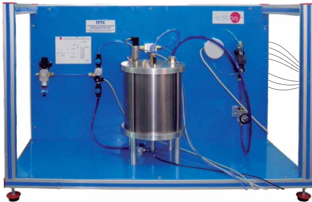
Unit: TFTC. Nozzle Performance Test Unit
