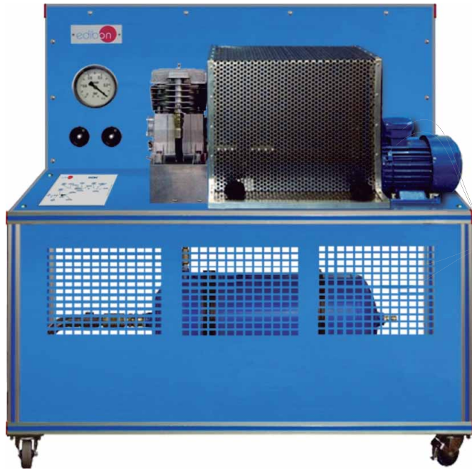
① Unit: HCRC. Reciprocating Compressor Unit
