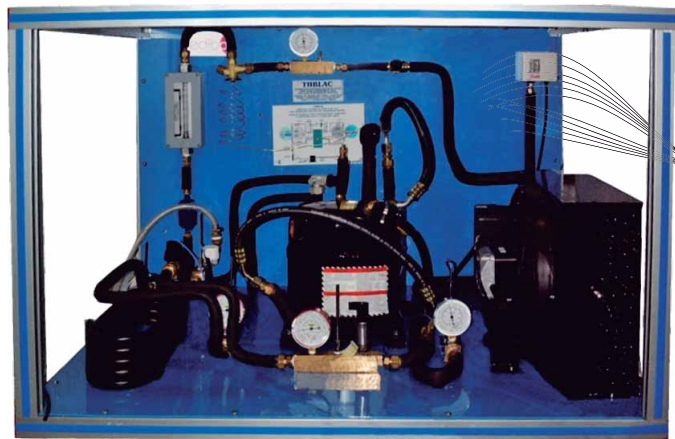
① Unit: THBLAC. Heat Pump Unit (one condenser (water) and one evaporator (air))
