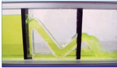
CFSDLC. Syphon spillway
