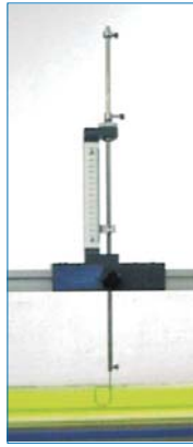
CFRMC. Level gauge for measurement of the water height (hook and point gauge)
