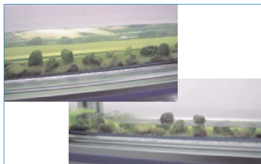
CFPLRC. Artificial roughened bed (3 different models)
