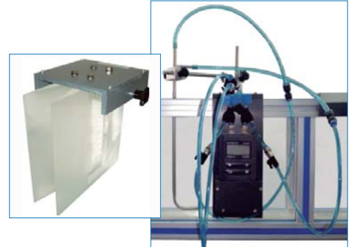
CFTVCC. Venturi tube, with pressure transducers, converter and differential pressure digital indicator for input flow measurement
