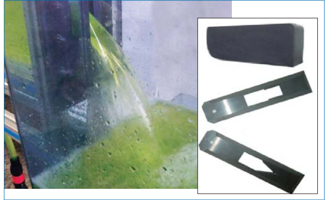
CFVDGC. Broad and thin crested weirs
