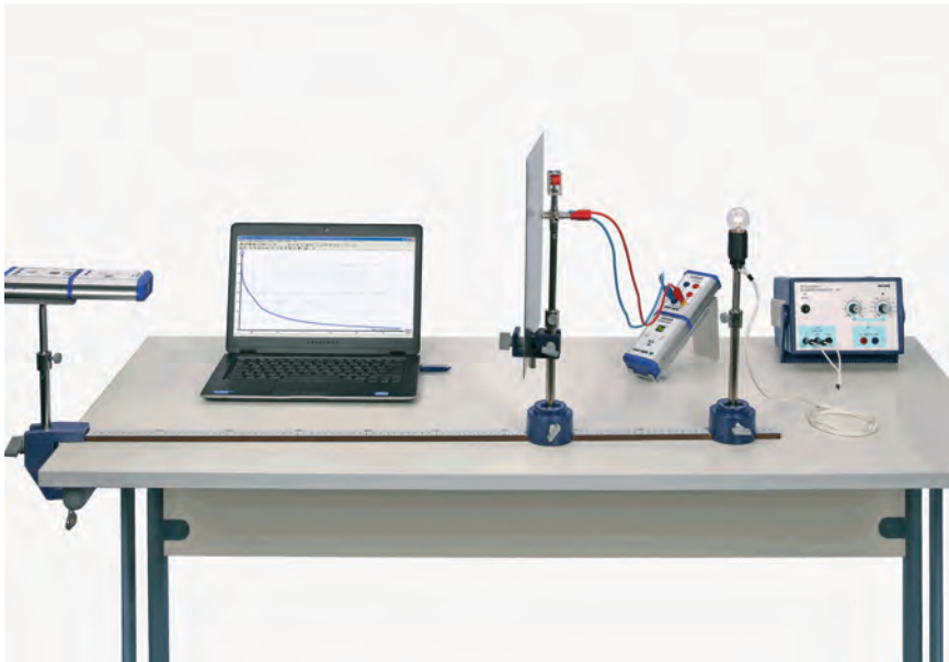
Luminous intensity as a function of the square of the reciprocal of the distance (lamp - diode).
