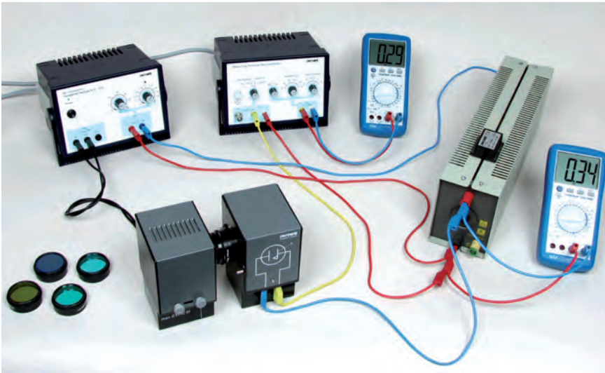
Photoelectric current intensity I as a function of the bias voltage at different frequencies of the irradiated light.
