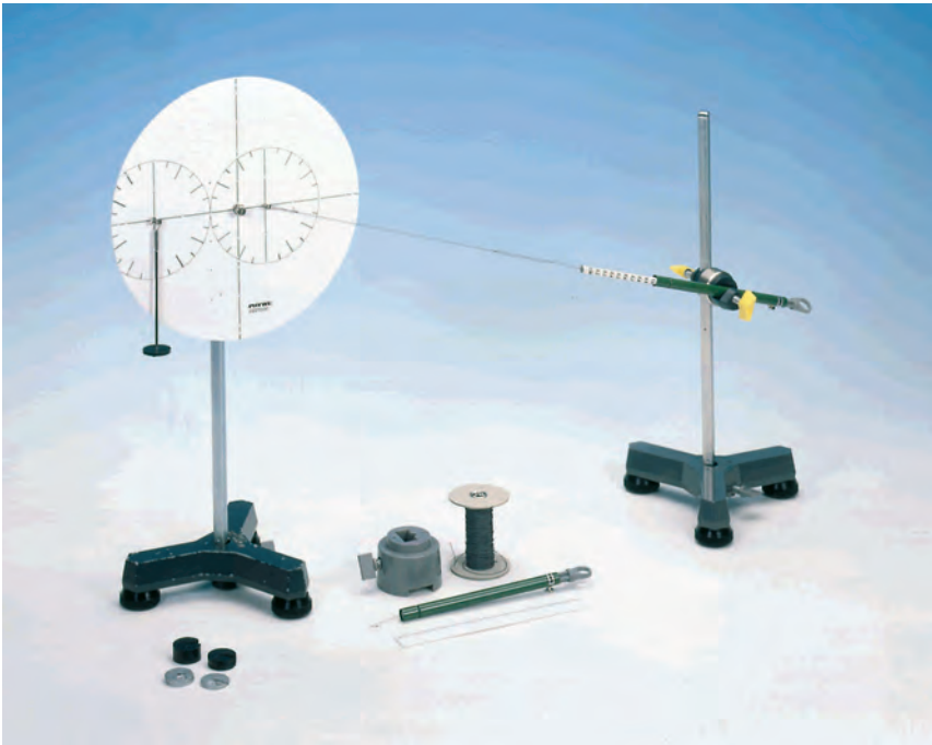
Moment as a function of the distance between the origin of the coordinates and the point of action of the force.
