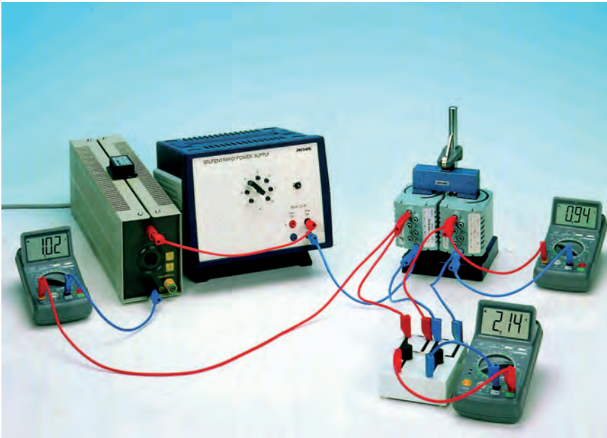
Secondary short-circuit current of the transformer as a function 1. of the number of turns in the secondary coil, 2. of the number of turns in the primary coil.
