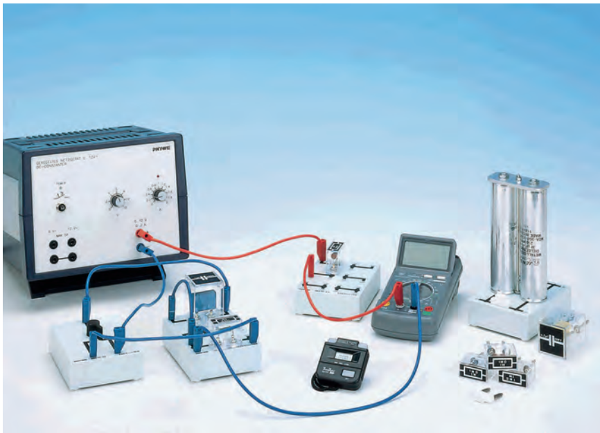
Course of current with time at different capacitance values; voltage and resistance are constant ( U = 9 \text{ V} , R = 2.2 \text{ M} ).
