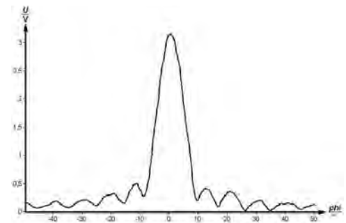
The angular distribution of the intensity of a plane ultrasonic wave diffracted at a slit.
