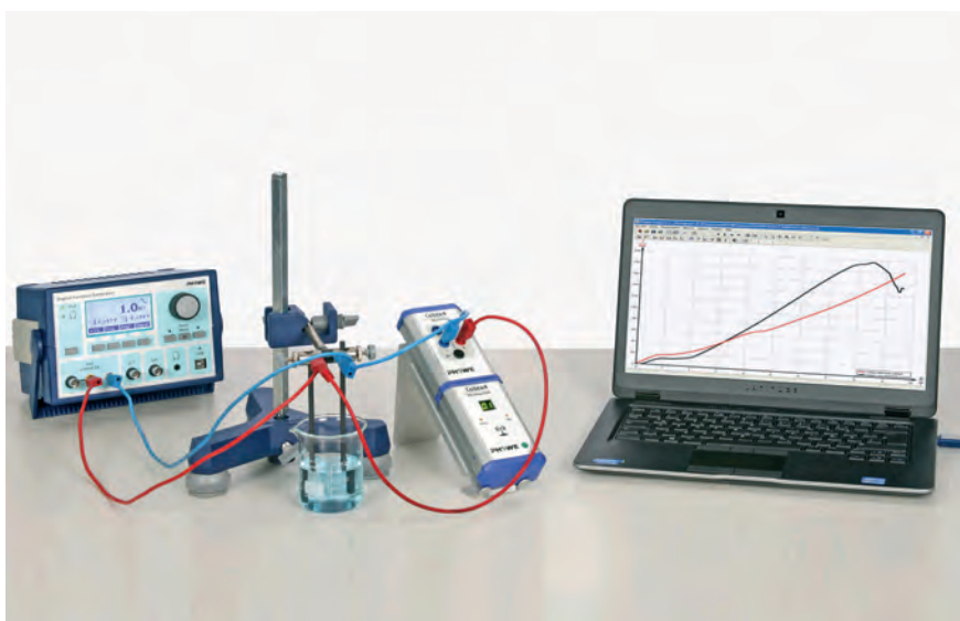
Current/voltage characteristics of an aqueous copper sulphate solution conducted with graphite electrodes and copper wires.
