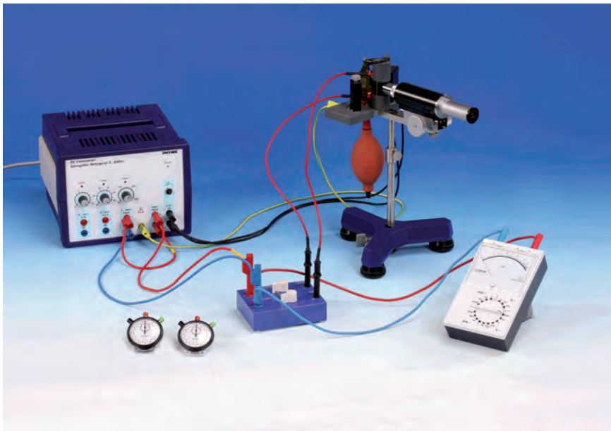
Measurements on various droplets for determining the elementary charge by the Millikan method.
