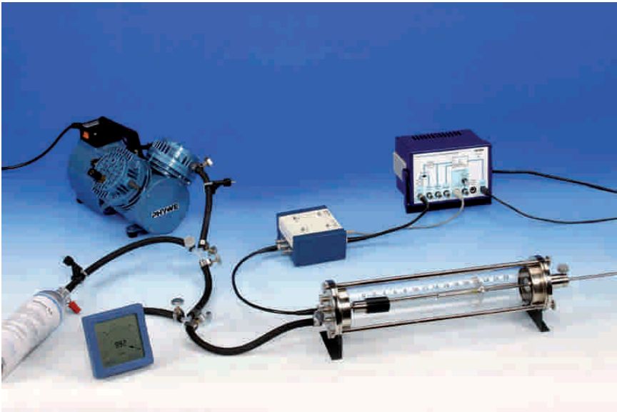
Influence of the type of gas on the energy loss of alpha particles.
