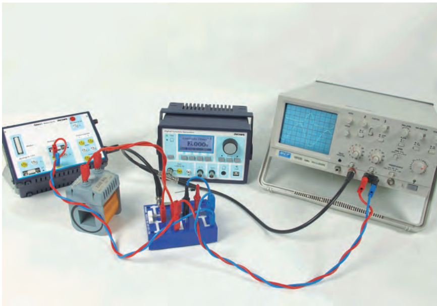
Voltage tapped off the diode at U_{SS}=9V . The circuit is oscillating chaotically.
