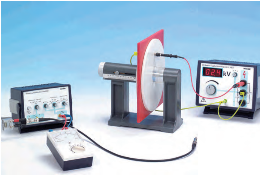
Electrostatic charge Q of a plate capacitor as a function of the applied voltage U_c , with and without dielectric (plastic) between the plates ( d = 0.98 cm).
