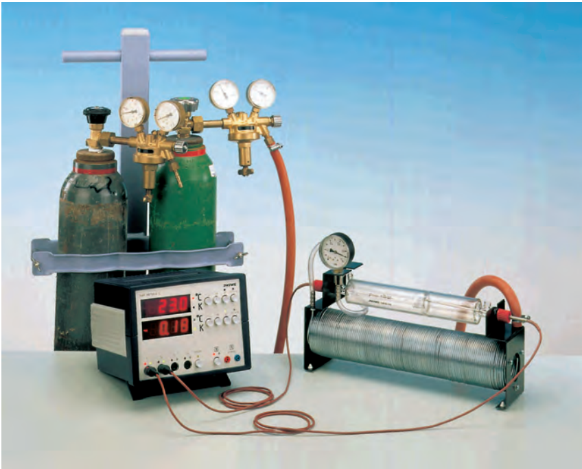
Temperature differences measured at various ram pressures.
