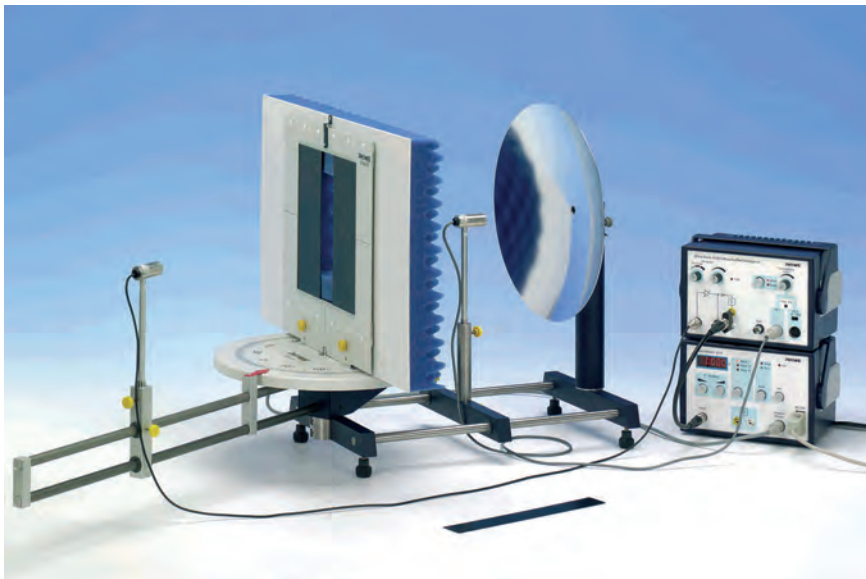
The angular distribution of the intensity of a plane ultrasonic wave diffracted at a slit.
