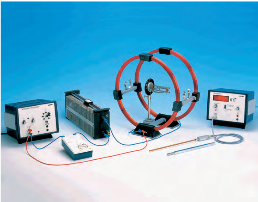
Linear function to determine the horizontal component h_{BE} of the magnetic flux density of the earth-magnetic field.
