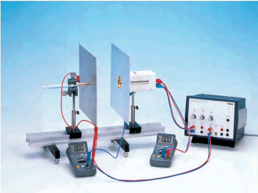
Electric field strength as a function of the plate voltage.
