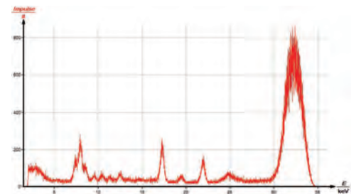
Characteristic fluorescence spectrum of the detector components (energy of the primary radiation E_0 = 32.5 keV).
