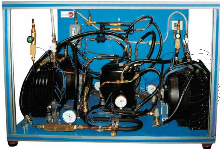
① Unit: THB22C. Heat Pump Unit (two condensers (water and air) and two evaporators (water and air)).
