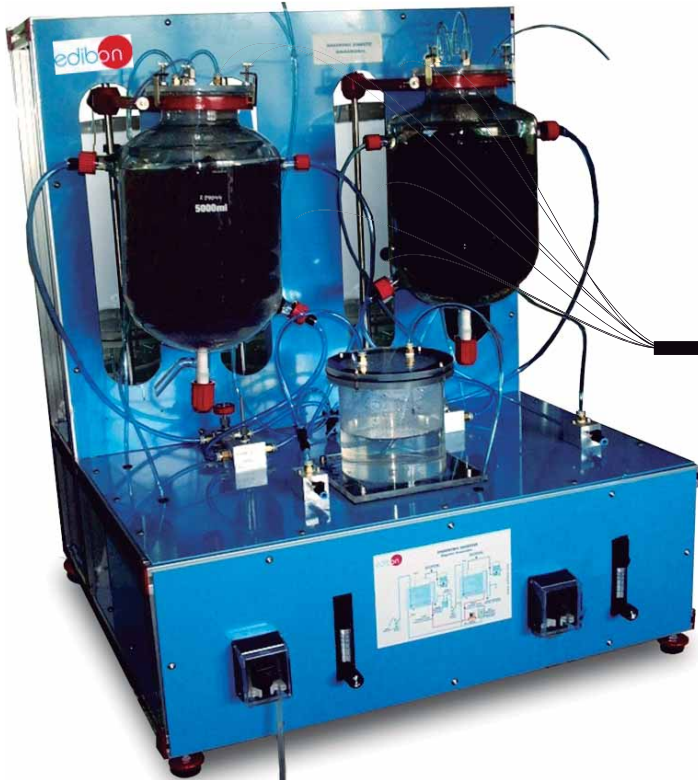
① Unit: PDANC. Anaerobic Digester
