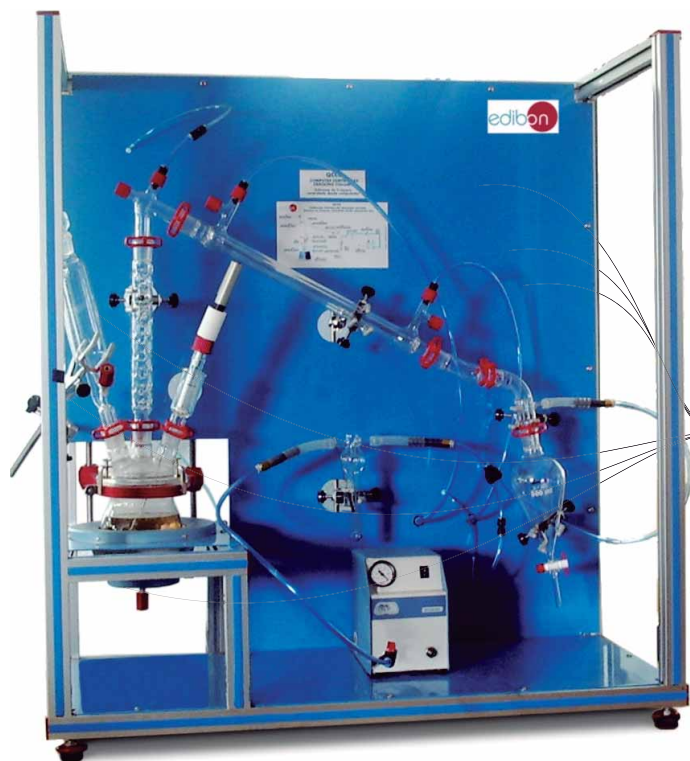
① Unit: QCCC. Cracking Column
