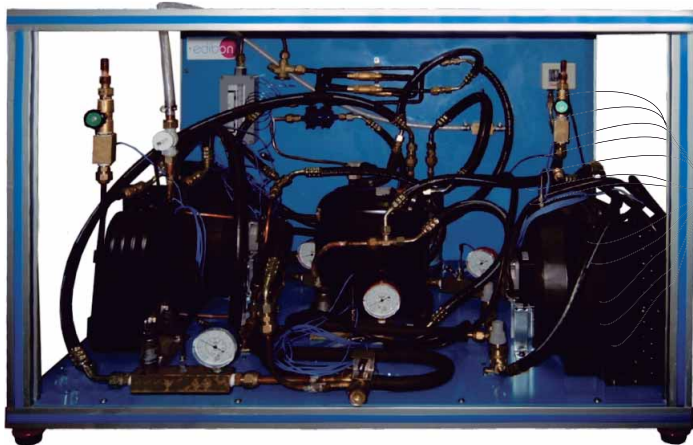
① Unit: THBA2C. Heat Pump Unit (one condenser (air) and two evaporators (water and air)).
