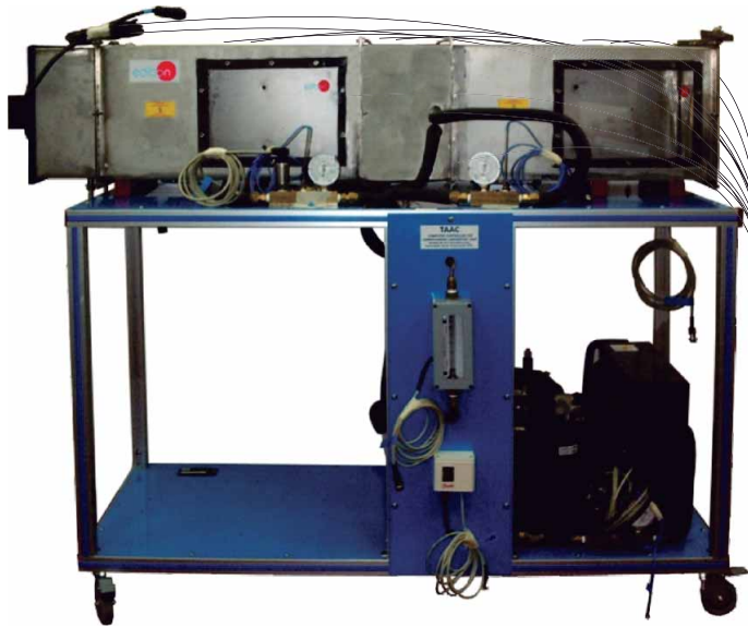
① Unit: TAAC. Air Conditioning Laboratory Unit
